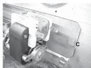
Attach the connectors from the black and red wires to the blower.
